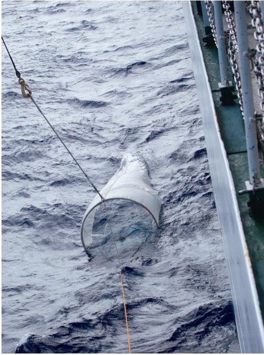
Fig. 2. ORI net towed on the surface of the western Pacific Ocean on the starboard side of R/V MIRAI (Cruise No. MR-06-05-Leg 3) at night at a speed of 2.5 knots, using a net that was 6 m long and with a diameter of 1.5 m
