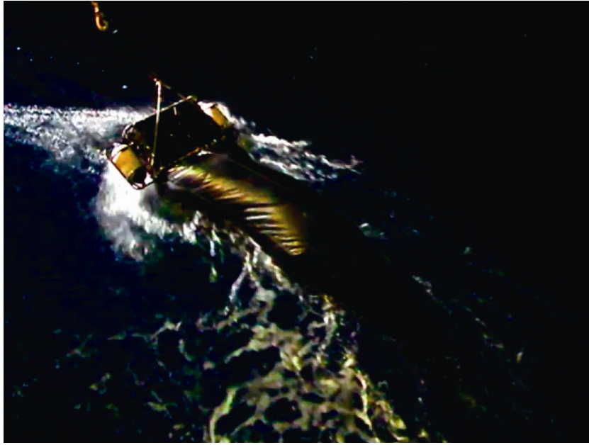
Fig. 3. Neuston net towed on the surface of the western Pacific Ocean on the starboard side of R/V MIRAI (Cruise No. MR-09-04) at night at a speed of 2 knots, using a net that was 6 m long and with a diameter of 1.3 m.
