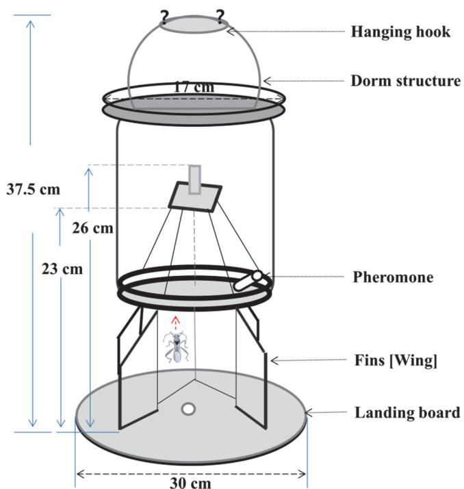
Fig. 1. Modified rocket trap with wing colors and landing boards along with dimensions baited with aggregation pheromone of *Riptortus pedestris* (Drawing: R. Maharjan)
